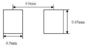
Note: Print solder in thickness of 0.08mm to 0.10mm
