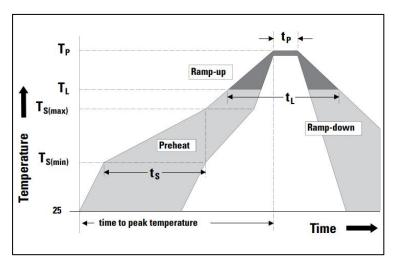
—All temperature refer to topside of the package, measured on the package body surface —If reflow temperature exceeds the recommended profile, devices may not meet the performance requirements
